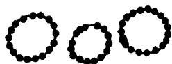
Figure 8 (PS/PVC) (1:1) blend with SbBgCHMA (20 wt %), as in Figures 4a and 7 , but annealed for 1 h at 200°C. The interfaces are covered by strings of micelles
